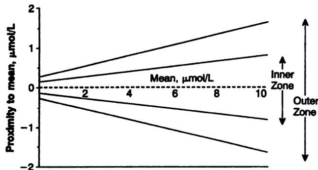
Fig. 1. Chart showing the inner and outer target zones in which the proximity of a result to the consensus mean ( $x - \bar{x}$ ) can be plotted.
